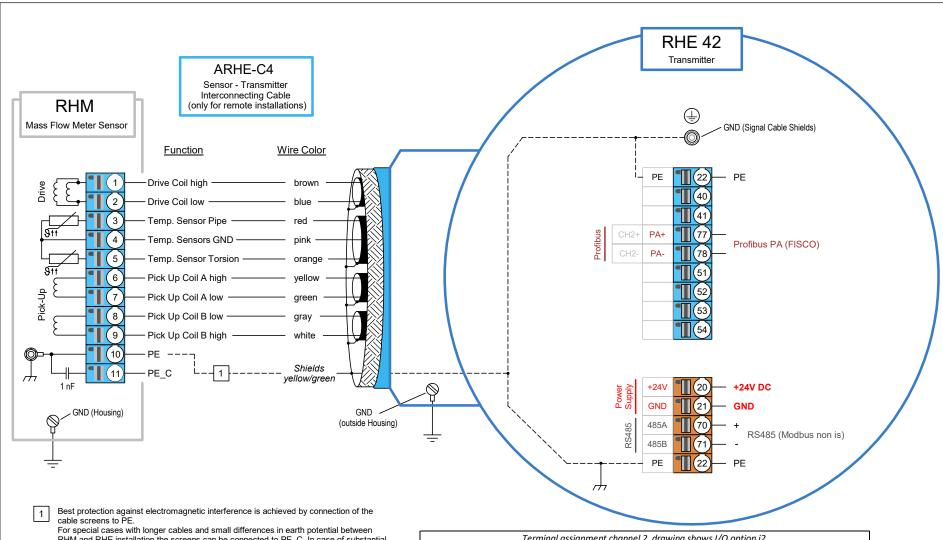
RHM and RHE installation the screens can be connected to PE\_C. In case of substantial potential differences a potential equalization cable is mandatory.
